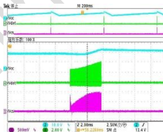
Output Open Protection Vin=90V Load=16*1W
